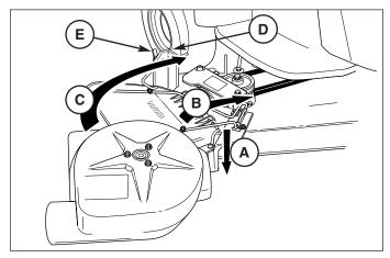
Figure 17. Install Turbo Blower
